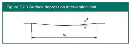
S2.2.4 Earlier intervention is required if the depression alone results in standing water wider than 500 mm or exceeding 1 m<sup>2</sup> in area, at 2 hours after the cessation of rainfall.
