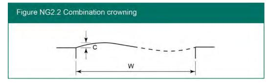
C is the Surface crowning contribution. If this value is greater than the combined defect intervention limit specified in Table S2.2, intervention is needed.
