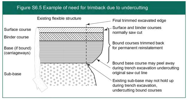
2) There may be no need for trimback when undercutting occurs if PMMA is used as sub-base and base. If an FCR or a FSMR (see A9) is used, then consideration of shrinkage during curing must be demonstrated to ensure support of the overlaying structure.
