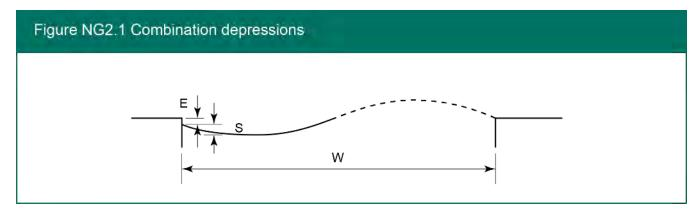
E is the edge depression contribution and S is the surface depression contribution. Once E and S are measured, they are compared with the combined defect intervention limits set in Table S2.1. If E or S is greater than the specified limit, intervention is needed.
