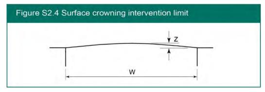
S2.2.6 Earlier intervention is required if crowning alone results in standing water wider than 500 mm or exceeding 1 m<sup>2</sup> in area, at 2 hours after the cessation of rainfall.
